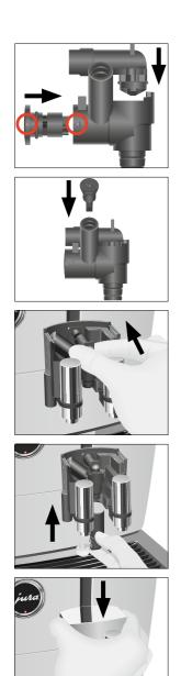
► Reassemble the milk system. When doing this, note the arrows on the individual parts (circled in red in the picture).
